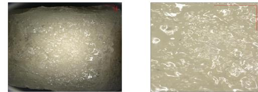
Microscope images of SMP foam coated with a poly(HEAAm) hydrogel and swollen with DI water at (top image) 20x and (bottom image) 1000x magnification.
