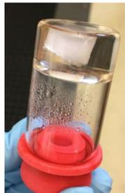
The pre-polymer was characterized by <sup>1</sup>H NMR and assayed in cell viability studies. The cross-linked foam was placed in a hydrogel solution and the hydrogel polymerized around and inside the pores of the foam. Hydrogel coated foams were characterized for their swelling ratios and shape memory properties.
