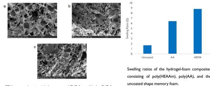
SEM images showing (a) the uncoated SMP foam, (b) the SMP foam coated with a poly(HEAAm) hydrogel, and (c) the SMP foam coated with an poly(AA) hydrogel.
